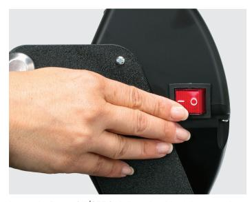
Locate the Power ON/OFF Switch on the side of the press, then turn the Power Switch ON.
