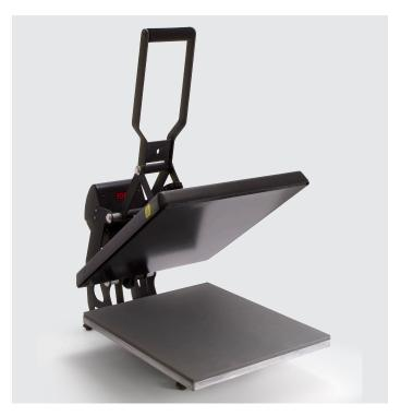
Locate the lift handle and position the heat platen in the UP (load) position.
