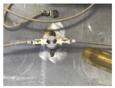
Using a heat gun or torch shrink the clear plastic heat shrink tubing around the connectors.
