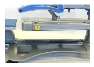
Lift the Heater off of the Lower Platen slightly using the Handles, pull out the Lower Platen, lower the Heater and adjust the Adjustment Knob until the Heater is at its lowest possible point to give maximum access in later steps
