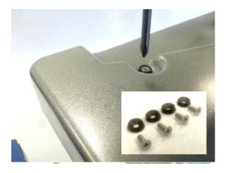
Unscrew 4x #10-24 x 5/8" Screws with Plastic Finishing Washers using #2 Philips Screwdriver
