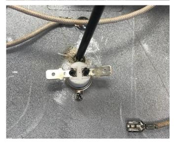
Unscrew the Selco From the Heater and remove the Selco that is no longer heating.
