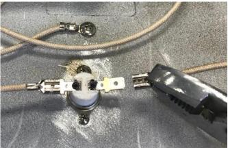
Remove the wires from the Selco.
