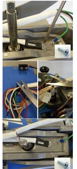
Remove TRIAC using #2 Phillips Screwdriver, saving #6-32 x ½" screw
