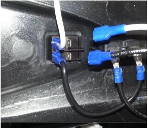
Unplug Black & White wires from Power Switch as shown to disconnect from Controller
