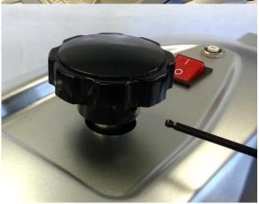
Replace Pressure Adjustment Knob, aligning set screw with flat of shaft and tightening with 3/32" Allen Wrench
