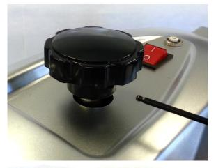
Loosen set screw in shaft of pressure adjustment knob and remove knob using 3/32" Allen Wrench
