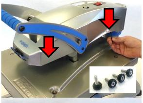
Replace housing onto press and insert 4 #8-32 x ½" Thumb Screws (right 2 shown), tightening with 9/32" Allen Wrench
