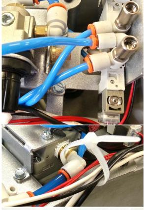
Route two top Swing Valve exhaust air hoses through bracket hole as shown
