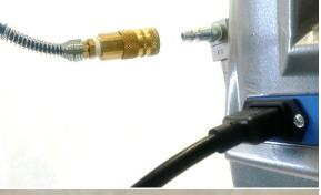
While heater is lowered, disconnect air supply line from air filter
