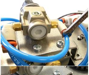
Remove 5/32" air tube from Mini Regulator by pressing down on push-to-connect fitting collar with 5/32" Combination Wrench or Needle-Nose Pliers while pulling out air hose
