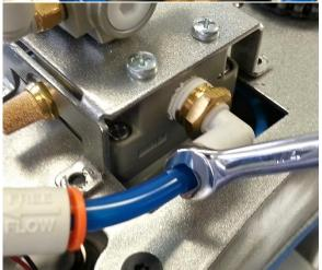
Remove 1/4" air tubes from Mini Regulator old EP Regulator by pressing down on push-to-connect fitting collar with 1/4" Combination Wrench or Needle-Nose Pliers while pulling out air hose
