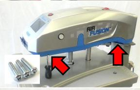
Replace Housing onto press and screw in three #8-32 x 3/4" Screws using Short #2 Phillips Screwdriver
