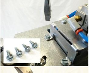
Lift up EP Regulator Cage by unscrewing 4x #8-32 x 1/2" Sheet Metal Screws from Pneumatic Package using Flathead Screwdriver or 1/4" Socket Wrench
