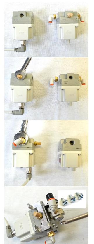
Unscrew power supply cord from bottom of old EP Regulator and screw onto new EP Regulator
