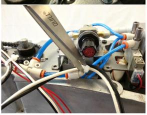
Cut Zip Ties on old EP Regulator fittings using Scissors
