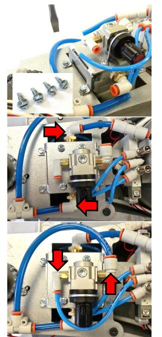
Attach EP Regulator Cage to Pneumatic Package by screwing in 4x #8-32 x 1/2" Sheet Metal Screws using 5/16" Combination Wrench
