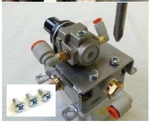
Remove old EP Regulator from Cage by unscrewing 3x M4 x 8mm Screws using #2 Phillips Screwdriver
