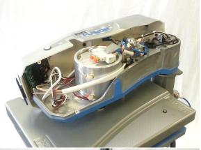
Lift off Control Housing and lay it gently on left side of press
